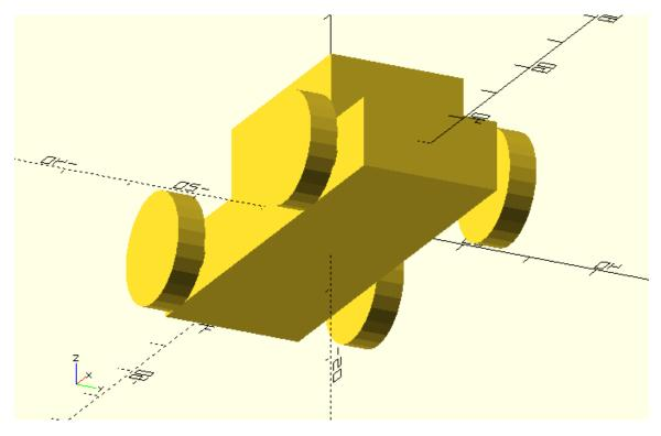
You should notice that a wheel is no longer created at the origin. You should keep in mind that the use command works like the include command with the only difference being that the use command doesn't create any objects, but rather just makes the modules of the external script available in the current script.
