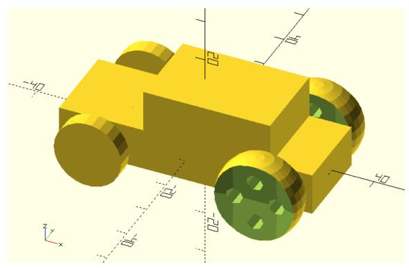
With this example it should be clear that the name of the script doesn't have to be the same as the name of the module as well as that a script can contain multiple modules. There is no right or wrong way on how you should go about organizing your library of modules. In the last example a wheel.scad script which defines the different wheel modules was used. Alternatively you could have saved each module as a separate \*.scad script.
