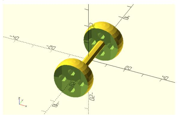
In order to create an axle with different wheels on each side, the definition of the of the axle\_wheelset module would need to be modified. Instead of referencing the first object, children(0), for both sides, the axle\_wheelset module would need to reference the first object, children(0), for one side and the second object, children(1), for the second side.
