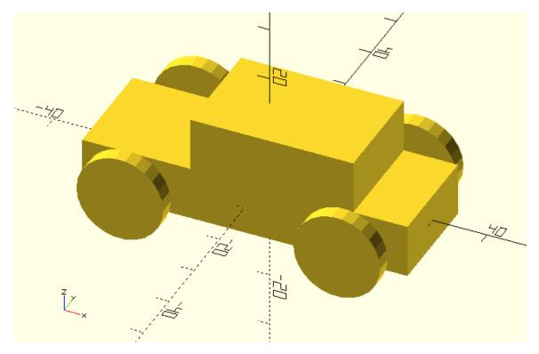
There are two ways in which the simple\_wheel.scad script can be utilized in your car design. It can be either included or used. To include the script, you have to add the following statement at the car's script.
