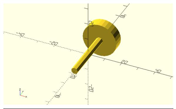
Add an axle\_wheel module on the vehicle\_parts.scad script. Make use of the children command to parameterize the specific choice of wheel design. Use the vehicle\_parts.scad script on another script to create any vehicle deign that you like.
